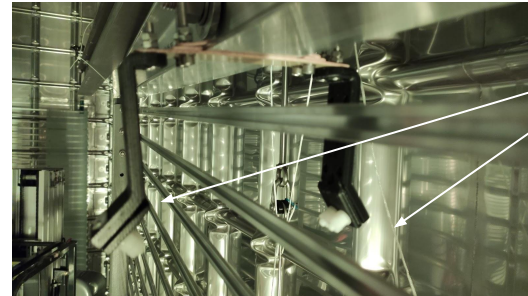
Fibers pointing towards cathode and membrane wall X-ARAPUCAs
