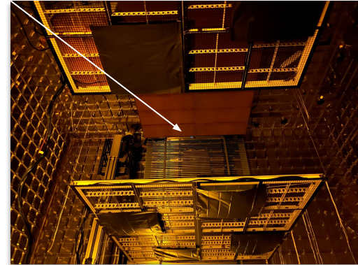
LED illuminated fiber pointing towards cathode X-ARAPUCAs
