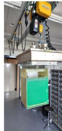
The cube TPC assembled and hanging on the top flange
