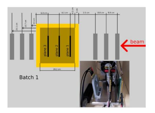
Cold operation for irradiated sensors – we reached -22C to -25C with two different T sensors used in different positions inside the box. A few (~4) voltage points per batch.
