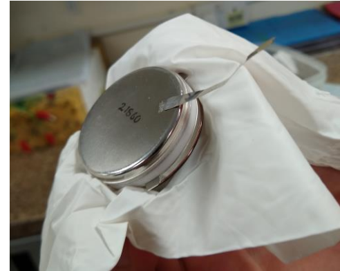
Bare MCP-PMT module (photo-cathode facing down)
