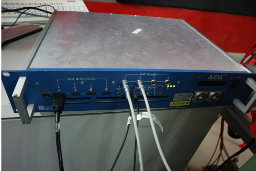
AIDA-2020 TLU connected to beam telescope
