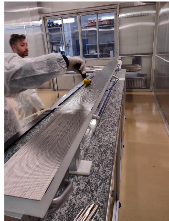
Stiffback-like technique for tube handling, gluing and positioning in the assembly tool
