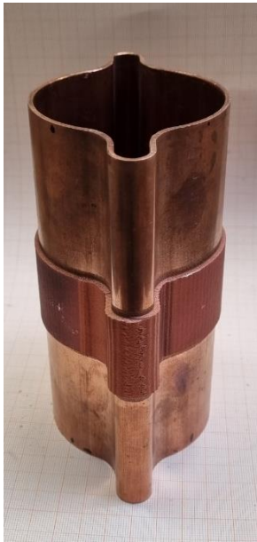
Chamber: 2mm layer sprayed all around
