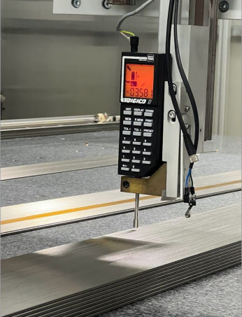
Semi-automatic system for planarity QAQC
