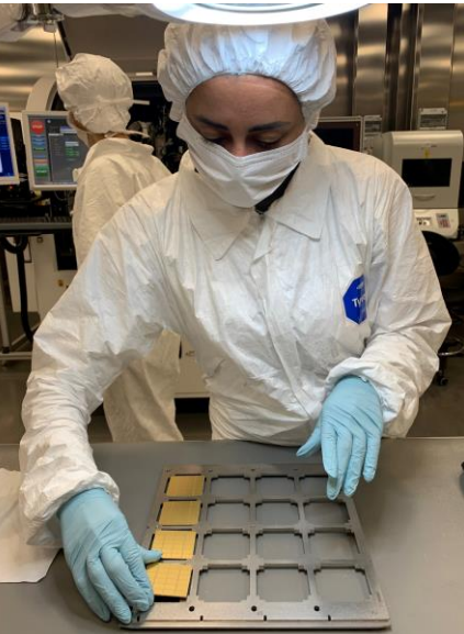
Frame holder for the PCBs each one to be assembled with 24 SiPMs
