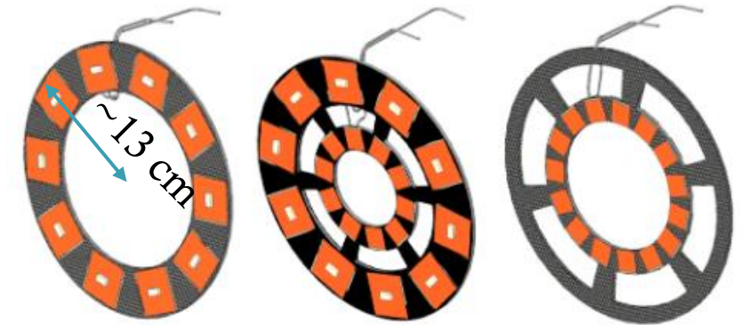
Inner system endcap rings (radius from ~5 cm to ~13 cm)
