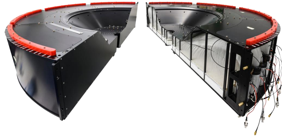
Fig. 4: FV0 – scintillator detector; 48 channels;
