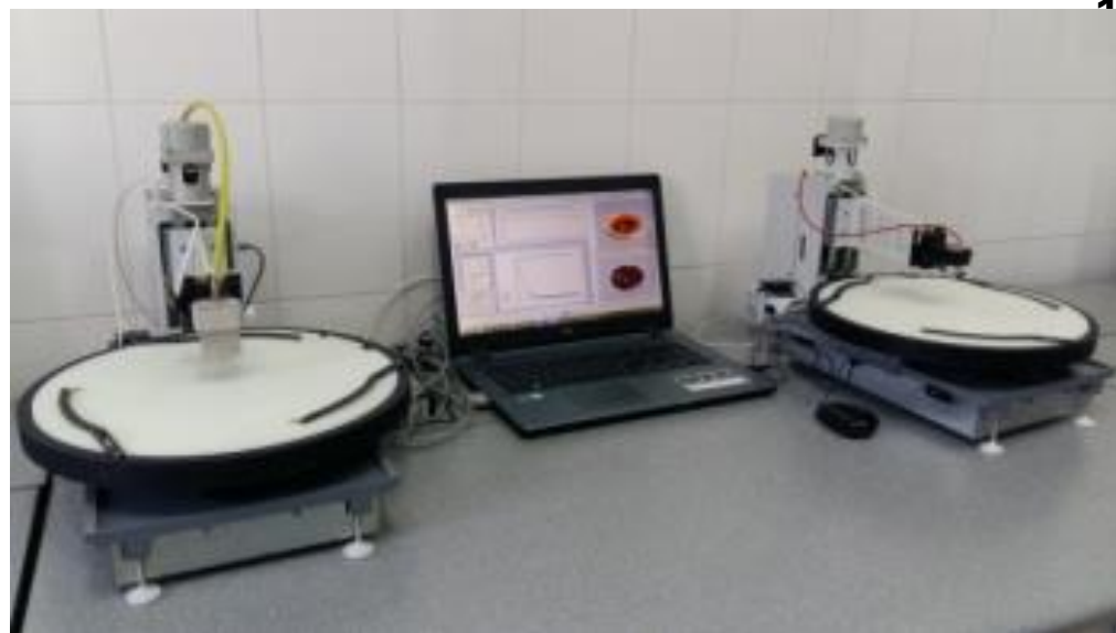
Figure 5 - Rometer instrument for measuring of electrical resistance and the device taumeter 2M to measure the lifetime of the minority carriers of silicon wafers.
