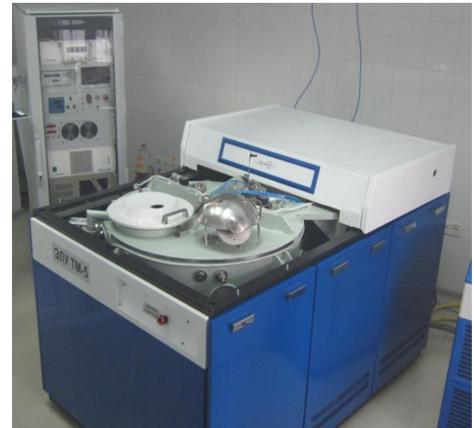
Electron-beam unit "ELU TM-5" for deposition of antireflective coatings on silicon solar cells
