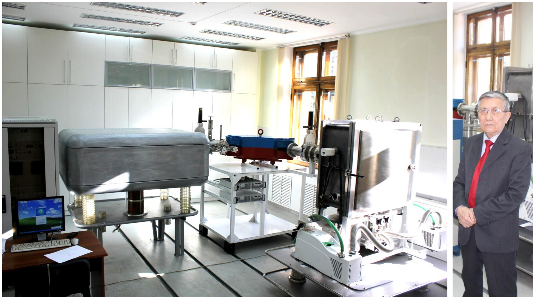
Figure 3 – Modernization of a unique accelerator of light and heavy ions, designed to create a p-n-junctions and growing of thick films by ion-beam deposition of low-energy ions. Entered into a preproduction of solar panels.
