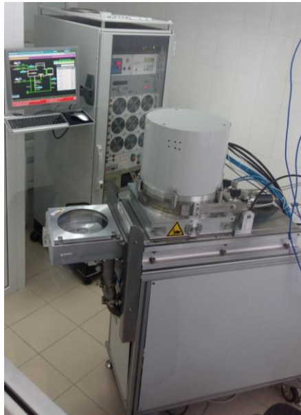
Upgraded the TM-200-01 MAGNA installation for deposition of nanostructures by magnetron sputtering
