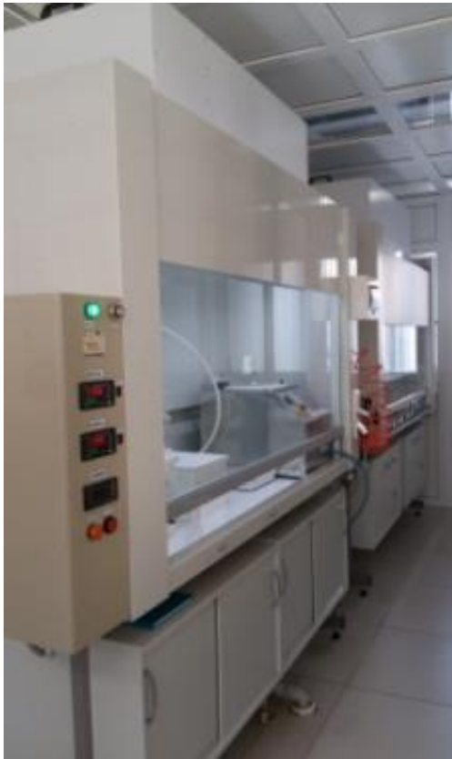
Figure 9 – Units for liquid chemical treatment in dimethylformamide and Caro mix in clean air with bath for remove of photoresist and DION-A003 for the production of pure water (18 MOm) in photolithographic technology
