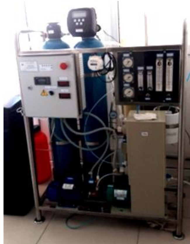
Figure 9 – Units for liquid chemical treatment in dimethylformamide and Caro mix in clean air with bath for remove of photoresist and DION-A003 for the production of pure water (18 MOm) in photolithographic technology
