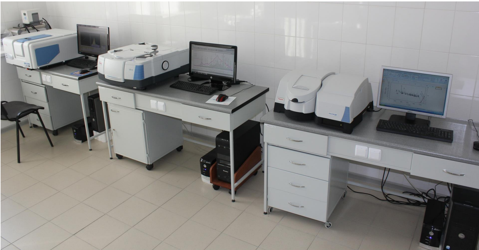
Figure 20 - Luminous spectrometer Lumina to determine the fluorescent properties of the films in the ultraviolet, visible and near infrared ranges.
