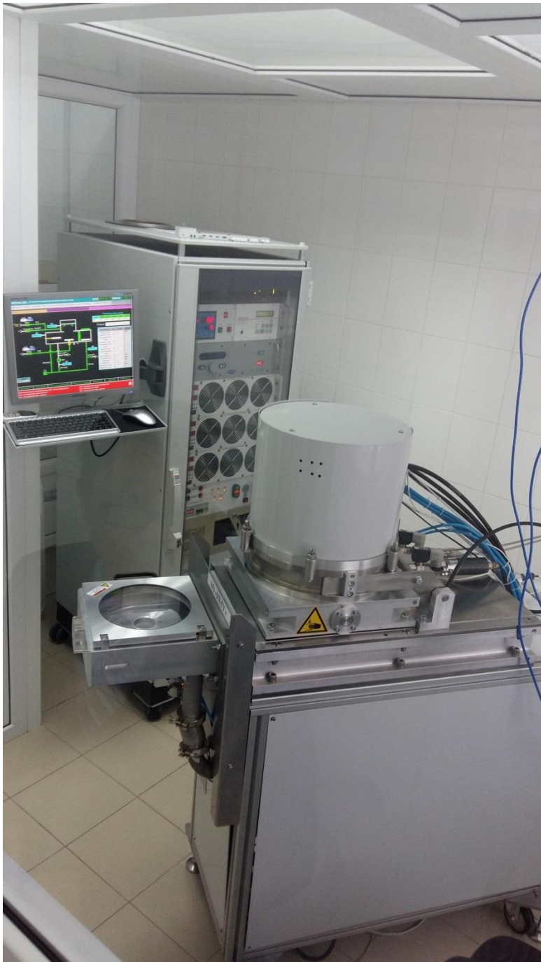
Figure 6 - Upgraded the TM-200-01 MAGNA installation for deposition of nanostructures and diffusion barriers on silicon wafers individually by magnetron sputtering
