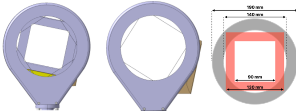
Figure 7 Left: old design (SPSBSAPB0030). Centre: new design SPSBSAPB0064. Right: schematic overlap of the old (red) and new (grey) aperture, illustrating the increased clearance for the beam passage.
