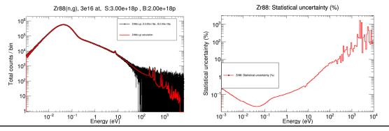
Background subtracted counts (left) and statistical uncertainty (right) for 100mCi  ${}^{88}Zr(n,\gamma){}^{89}Zr$  with  $3 \times 10^{18}$  protons on target for the sample and  $2 \times 10^{18}$ protons on target for background measurements.
