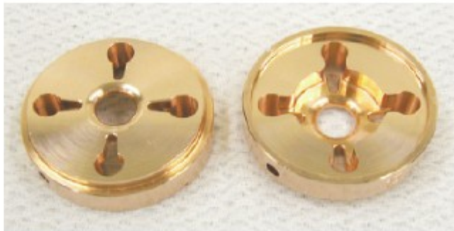
H-Series Cells Illustrating "Pie" Shaped Slots to Damping Manifolds
