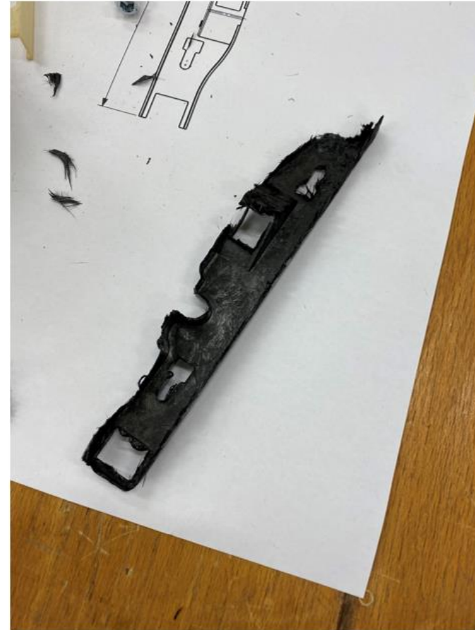
2 nd trial: too much material & improper closing
