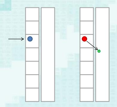
Recoil implantation followed by alpha decay, alpha particle stops within DSSD. Full energy deposited.
