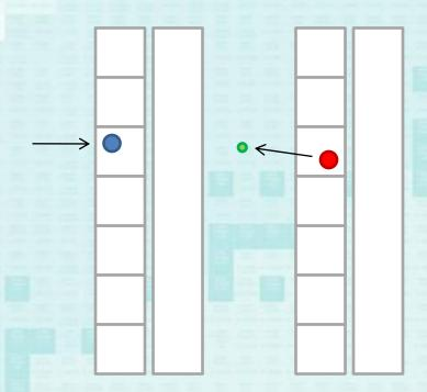
Recoil implantation followed by alpha decay, alpha particle escapes DSSD. Partial energy deposited.
