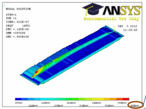
I added then that I needed to let the ANSYS calculation go on, after the beam has hit the spoiler, to see if there would be any stress build up that could reach fracture levels. And...
