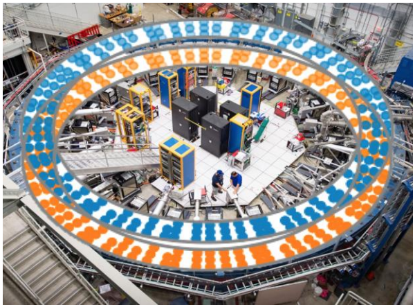
Fixed probes above/below muon storage region
