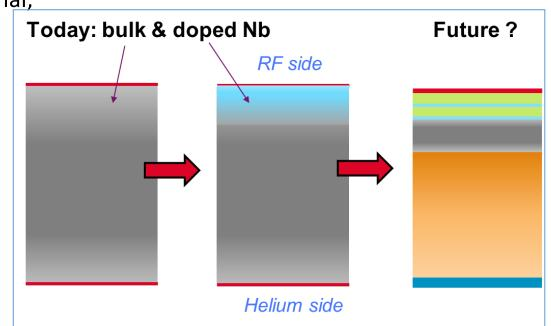
*Future : totally functionalized material, each layer its own role (thermal conductivity, high superconducting performance, multipacting mitigation....)*
