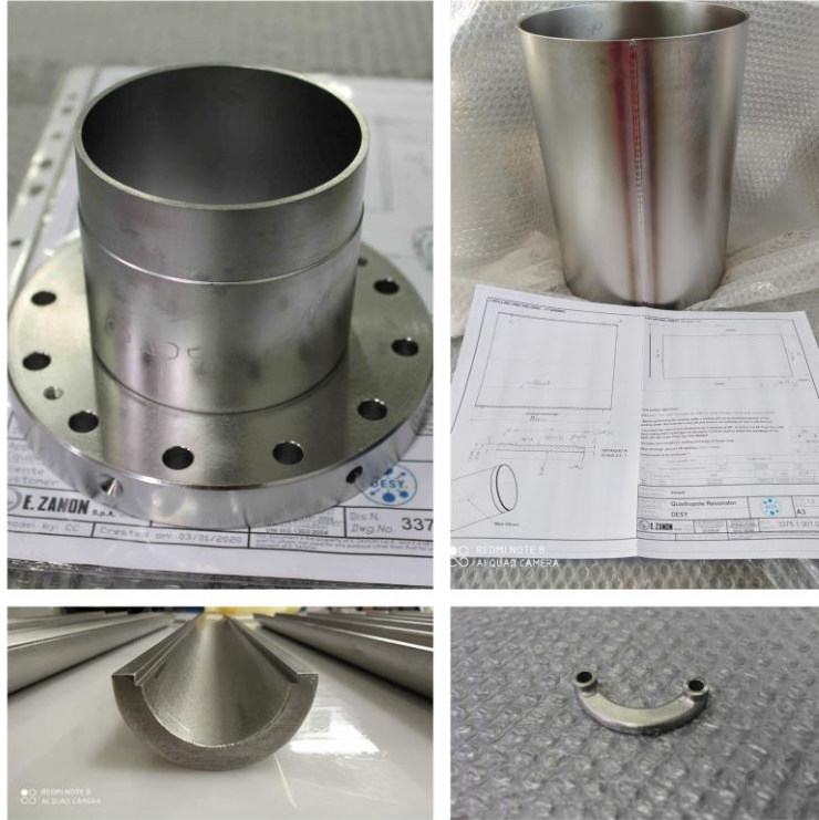
Cutoff tube, vessel, rods, and pole shoe before welding.
