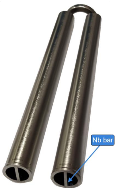
Metal bars welded to the rods to enhance their rigidity.
