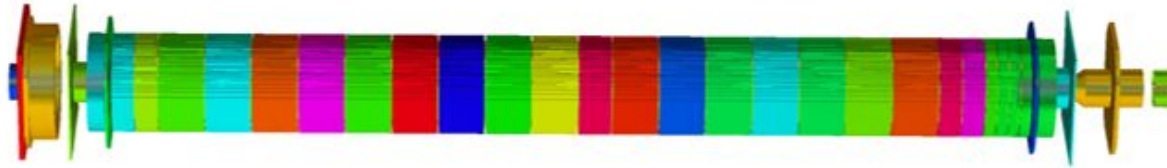
3D view of the RFQcb modelled in SIMION. The different colors refer to different potentials.
