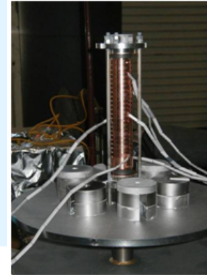
Pressure: 60 PSI (60 LB for this structure disks) Holding for 1 hour at 1020°C
