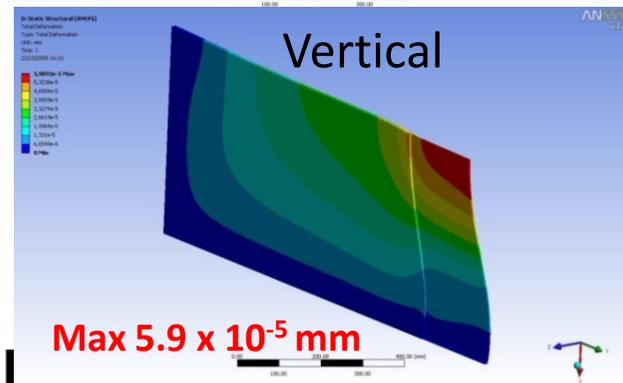
Deformation under its own weight as a function of storage orientation
