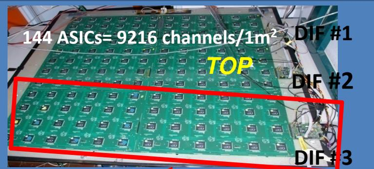
Every two ASUs connected to each other and connected to one DIF (Detector InterFace) card.
