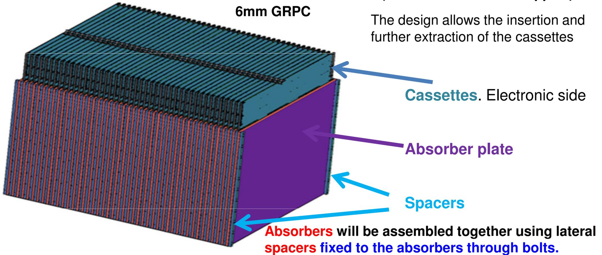
The **dead spaces** have been minimized as much as possible taking into account the mechanical tolerances (lateral dimensions and planarity) of absorbers and cassettes to ensure a safe insertion of the cassette.
