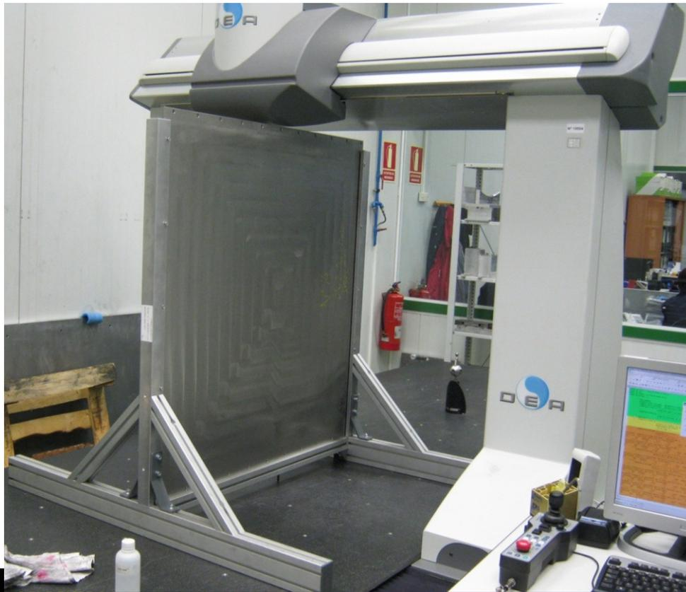
Planarity and thickness measurements (#49 points) performed by the company in vertical on both sides
