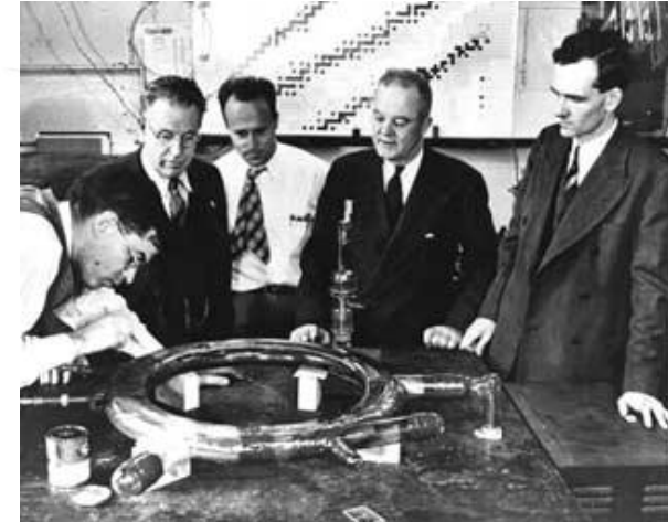
Scientists around the vacuum chamber of a 1947 General Electric synchrotron (photo courtesy of NSLS, Brookhaven)
