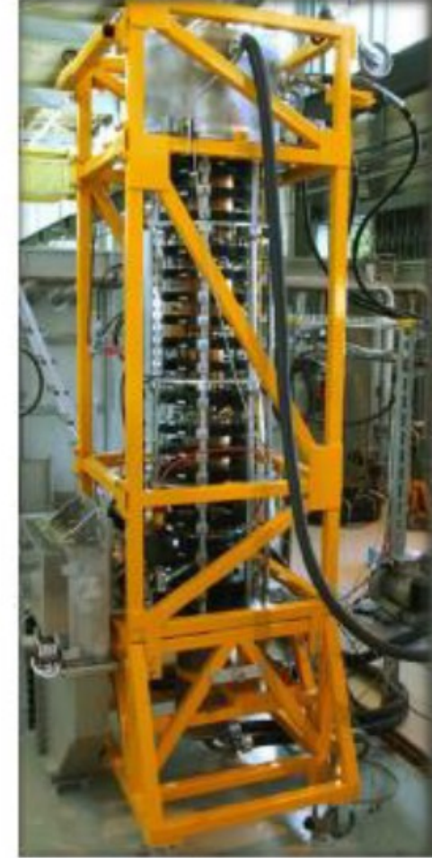
CERN LHC: 400 MHz, 300 kW, CW, \eta 62%
