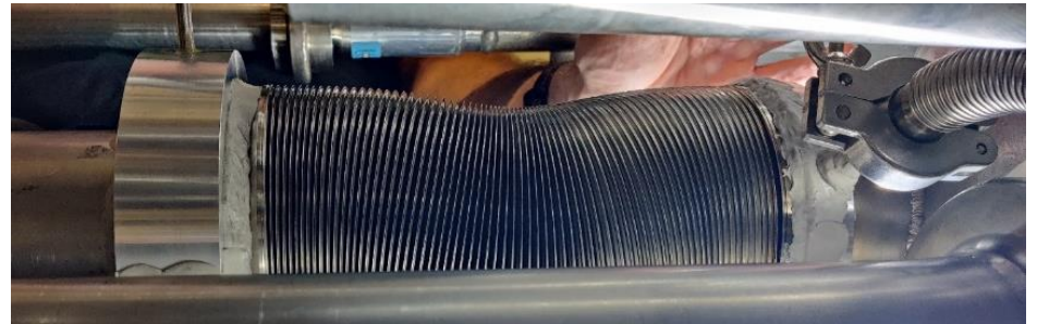
M2 bellows with 0.5 barg in the cold mass
