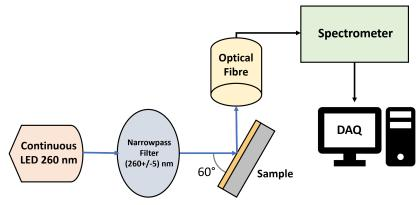
Schematic diagram of the apparatus used to take same side emission spectra.
