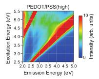
Fluorescent emission of Clevios under different excitation energies. Figure from Koyama et al [5].
