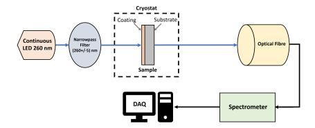
Schematic diagram of the apparatus used for emission spectra.
