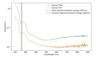
Absorbance spectra of Clevios coated Fused silica samples. Vertical lines are the excitation energy used for time resolved (267nm) and emission spectra (260nm)
