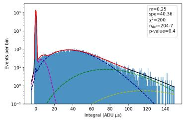
Integral histogram from the thick Clevios sample. Fit has been done to determine the Single Photo Electron (SPE) value.
