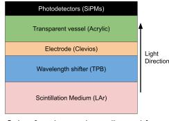
Order of coatings on the acrylic vessel for DarkSide-20k. Layers not to scale.
