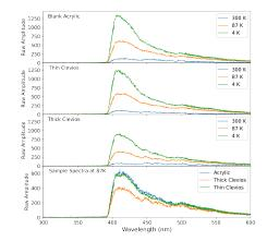
Emission spectra for blank acrylic, thick Clevios, and thin Clevios at 300K, 87K and 4K.
