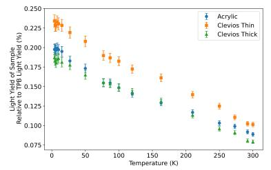
Light yield of each sample's fluorescence relative to TPB as a function of temperature.
