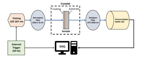
Schematic diagram of the apparatus used to take time-resolved measurements
