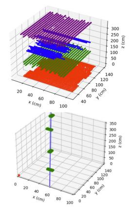
Cosmic ray events in the UVic MATHUSLA prototype, and a reconstructed muon track passing through all four layers
