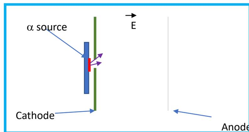
$\alpha$  energy altered by distortion of electric field near hole and possible interaction at the edge of the hole
