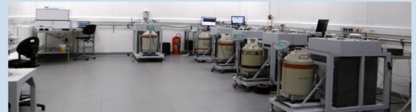
BUGS (UG): A range of HPGe detectors and alpha particle detectors for intrinsic and surface radioactivity measurements.
