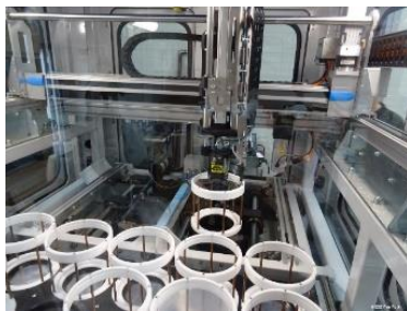
Automatic system for changing of samples for HPGe detectors (NUVIA company)
