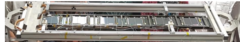
First ladder fully equipped with 12 functional 2S modules
