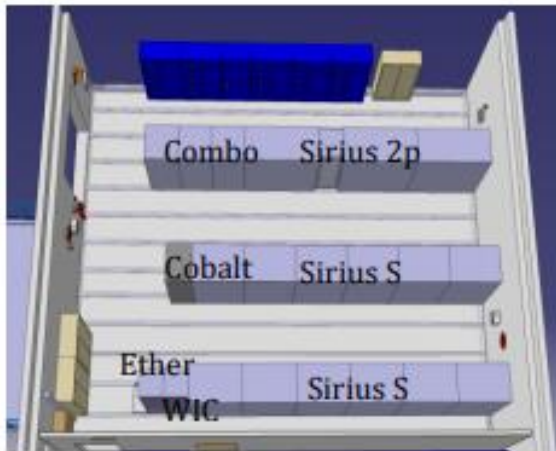
Figure 7 — Building 197/1-401: possible integration of SIRIUS converters.
