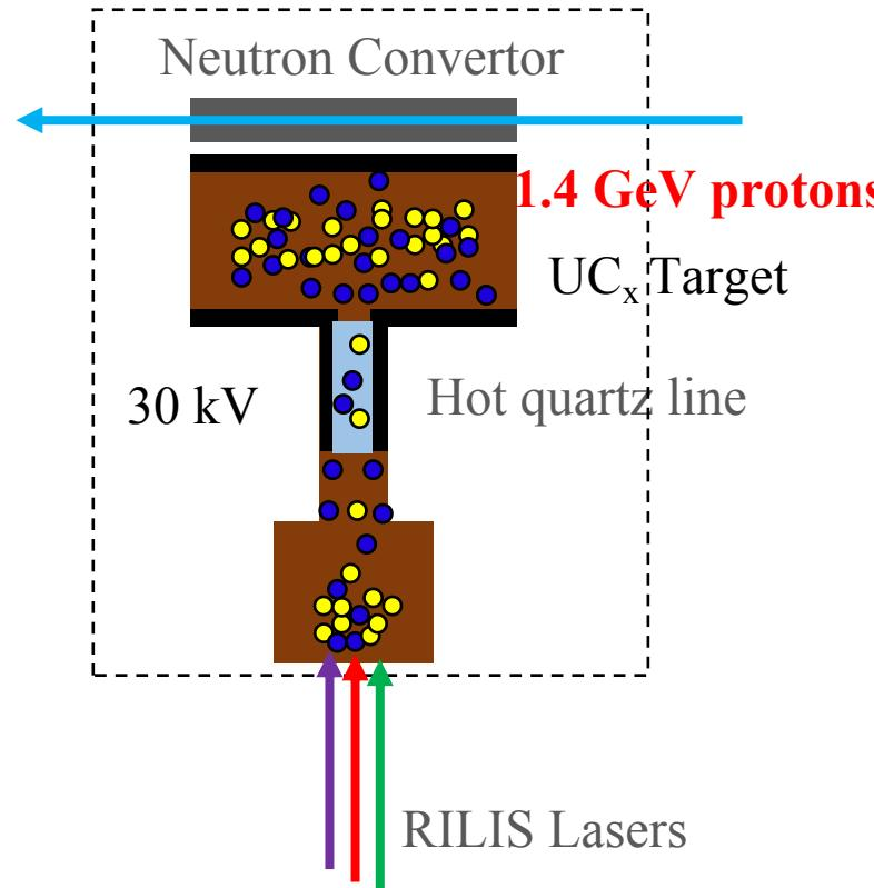
In Zn run, the ISOLDE target group combined the **neutron convertor**<sup>[1]</sup> and **hot quartz line**<sup>[2]</sup> to suppress the Rb background
