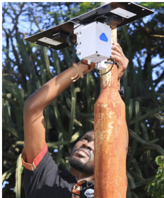
AirQo Binos: PM 2.5 , PM 10 , T, RH, P airqo.net
