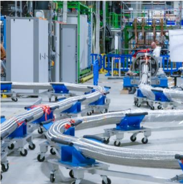
A novel, flexible cryostat, colloquially known as the "python", composed of 19 high-temperature magnesium diboride superconducting cables that can carry 120 kA. (Image: CERN)
