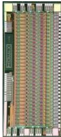
IdefX-Eclairs: 32 channels. Multiplexed outputs. 1 Range 200keV <3mW/ch
