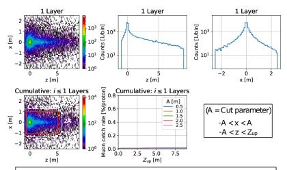
Making the system smaller does not signif cantly reduce the capture rate
