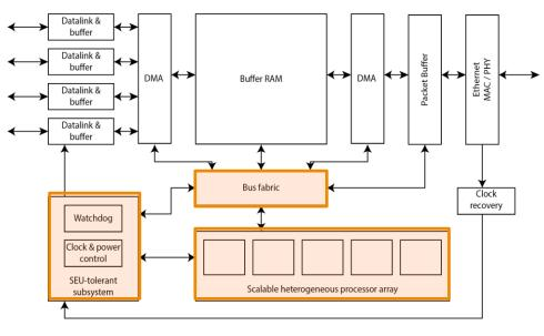
Proposed common interface ASIC for detector
