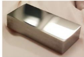
Polished block of Invar mimicking a connector
