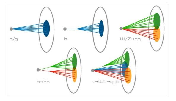
Jet structure indicates type of original particles
