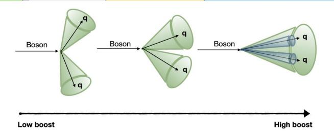
With high boost, two jets originating from single boson merge into single large jet. Probing jet substructure can improve signal sensitivity from QCD background.
