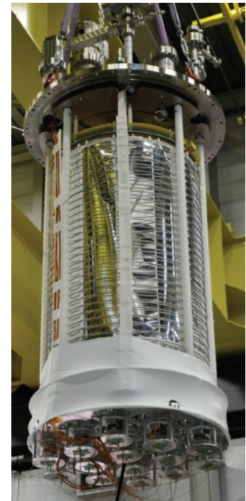
1t liquid Ar detector presently assembled at CERN
