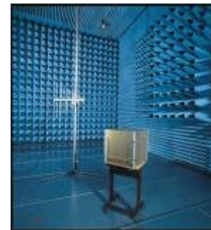
An “EMC”-enclosure reduces the emission level and increases the immunity against noise
