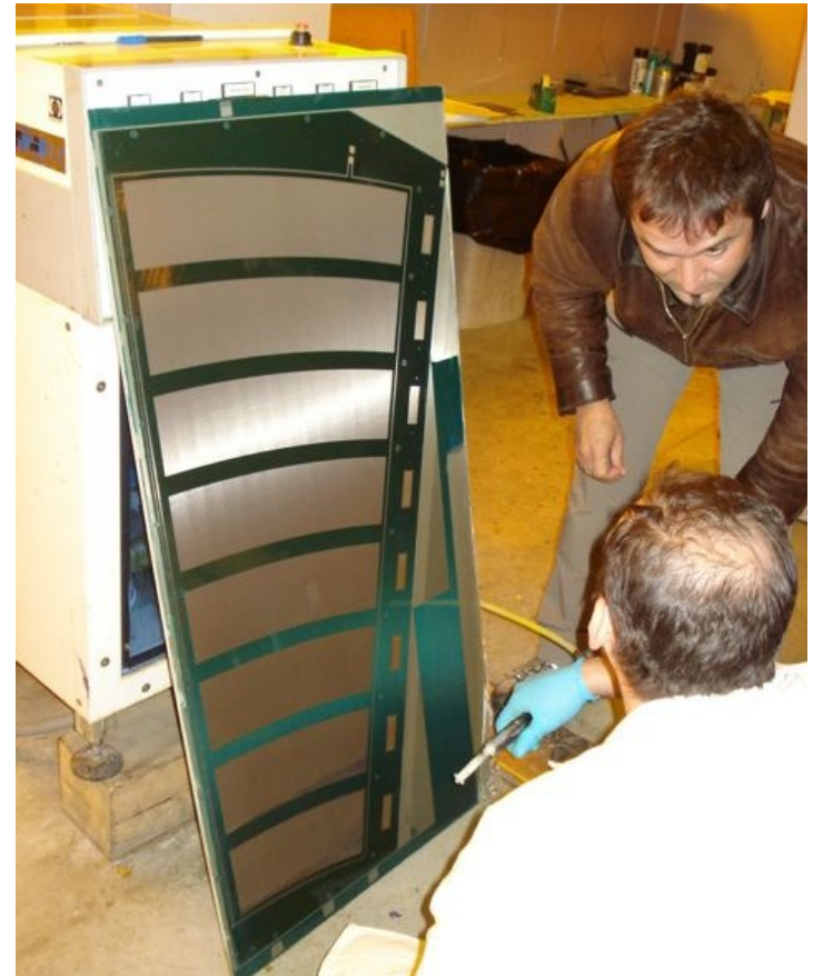
Chamber after pillar development but before curing
