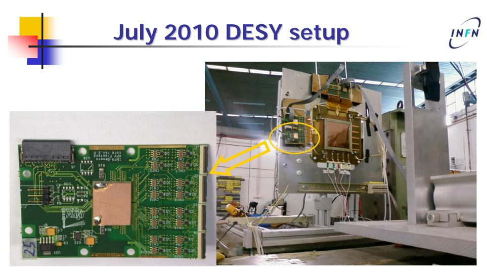
Small (10 x 10 cm<sup>2</sup>) chamber Only 4 APV cards + 1 ADC card (not shown) Flat cable ribbon connection
