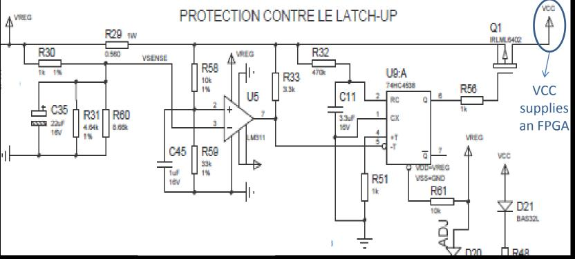
This card is installed, it has been tested under radiation, in one case the component U9 (L4931CD25) has failed at  $2x10^{11}$  p/cm2 (corresponding to TID 100 Gy).
