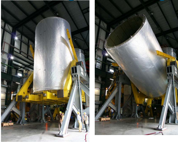
Vacuum Tank welded (Nov-Jan)
