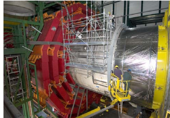
Coil Cooled to 4.5K in 25 days (Feb). Test on Surface (May-Aug)
