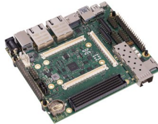
Custom hub PCB Interface between SoM and sensor layers/TLU
