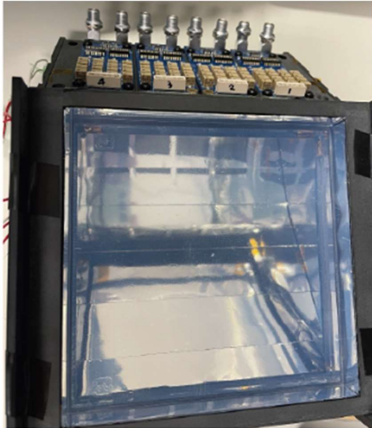
Real Cherenkov detector for J-PARC experiment
