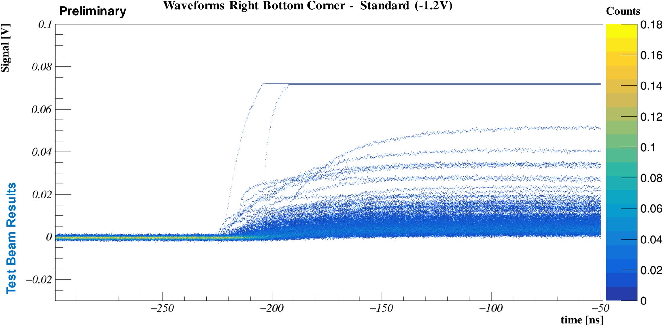
Waveforms with most probable value of deposited charge carriers appear more yellow
