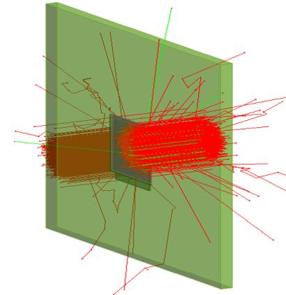
Particle beam passing through a single sensor in Allpix<sup>2</sup>
