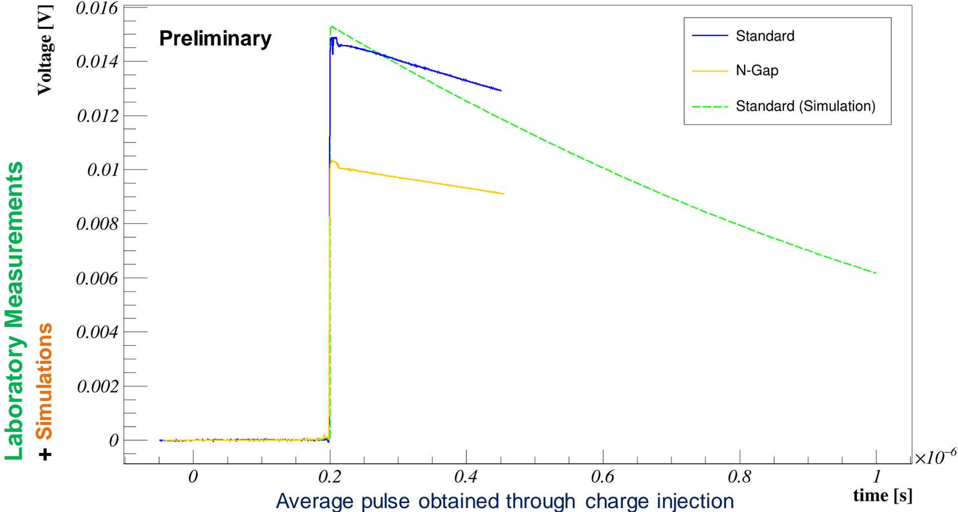
\*Difference in slope due to differences in how the reset current is distributed between simulation and APTS
