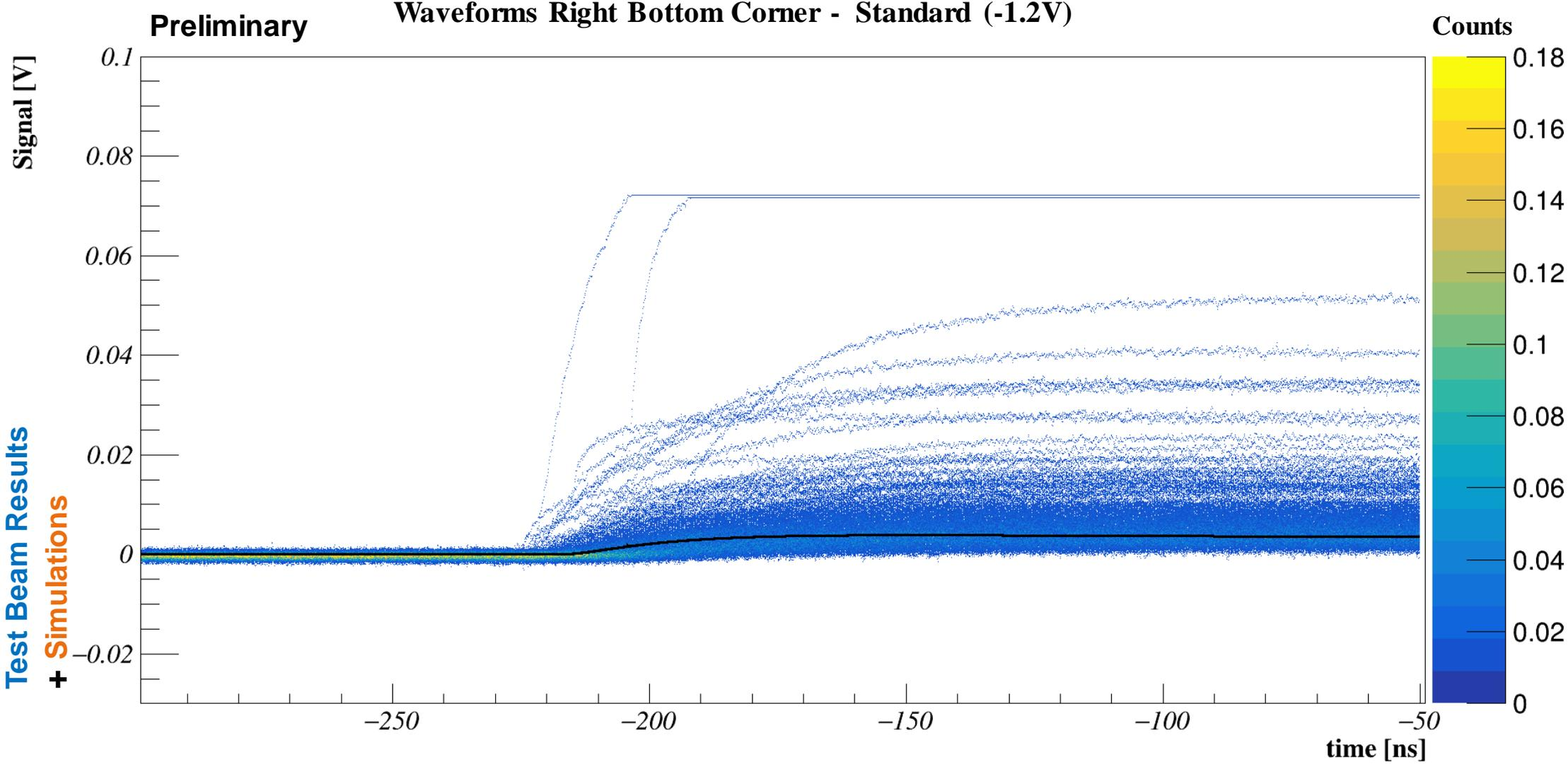
Simulation using most probable value of deposited charge carriers in black
